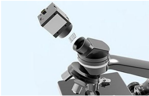
Schematic illustration on the location with the Smartlens is placed within the optical instrument (in this case a microscope) (Image credit: Marc Montagut)
